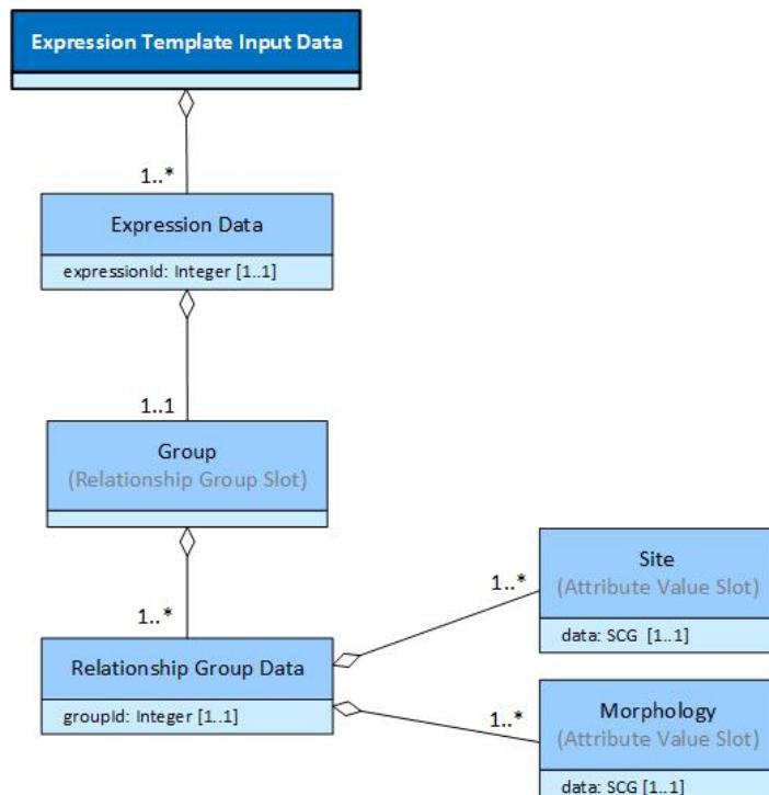
**Figure 7.1-5: Logical model of example 4 input data**
